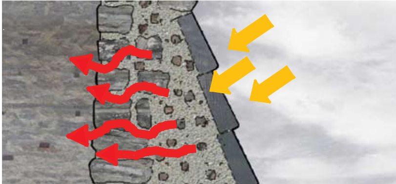
Figure 45 Dense masonry walls, a common thermal mass element on heritage buildings. Rubble wall study illustrating air and moisture movement through a heavy masonry wall. It is critical to maintain air and moisture behaviour characteristics to avoid creating unintended issues. East Block, Parliament Hill, Ottawa, ON. Source: MTBA Associates Inc.
