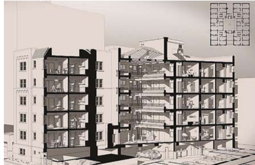
Figure 60 Building section explaining the interior arrangement in three dimensions, highlighting the enclosed central courtyard, which improves natural light and ventilation at no energy cost. The Blackburn Building Apartments (Somerset Street), Ottawa, ON. Source: The Blackburn Building (Darcy Charlton)
